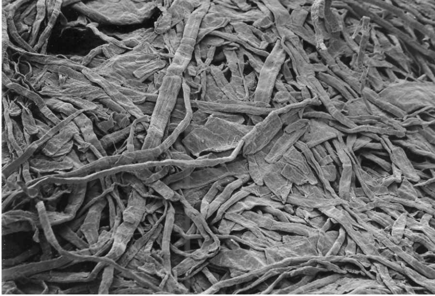
Figure A.2. S.E.M. of Bleached Wood Pulp at 150X Magnification
